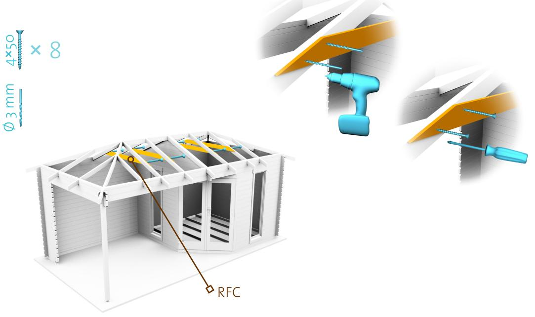
PLACE THE FIRST ROOFBOARD FLUSH WITH THE END OF THE PURLINS AND ATTACH WITH SCREWS
