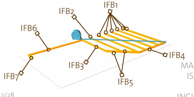
MAKE SURE THAT THE FOUNDATION IS INSTALLED ON A LEVEL SURFACE. CHECKING ALL DIRECTIONS, INCLUDING CORNER TO CORNER. 3%
