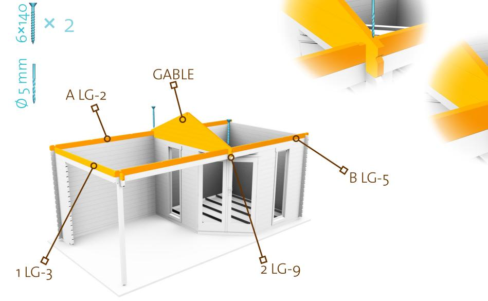
ATTACH TOP LOGS INTO JOKKMOKK 40 WALL LOGS WITH SCREWS. Ø 5 mm 6×140 × 44 ATL 3 TL •3 TL-4 00 **v** B TL-1 1 TL ♥ B TL-5 B TL-3 B TL-3 BTL-4 1 TL-4 BTL-4 BTL-5 BTL-2 16/28 58%
